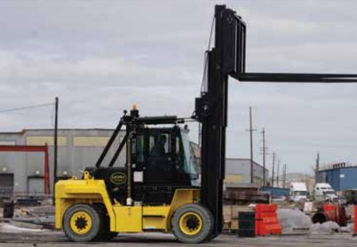
The RT features full-time all-wheel drive with heavy-duty planetary drive and steer axles and hydrostatic 2-wheel steering to maneuver through the most demanding applications.
