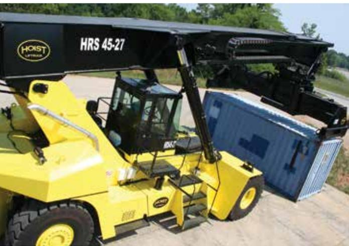
Some of its features include a cab capable of independently powered movement for superior operator visibility; inclination and optical distance sensors; and robust boom and attachment structure designed for 1 million cycles. The RS Series includes models and options to accommodate several applications, including front stabilizers for second- and third-rail operations as well as wide twist-lock, pin-style and trailer attachments.
