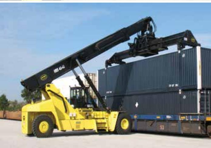
Several safety precautions are set in place for reliability and peace of mind. In case of power loss in the middle of lifting, the cab's rear window easily opens for emergency exit. An interlock safety system ensures proper locking sequence and overload warning system protects against lifts too heavy for the forklift.
