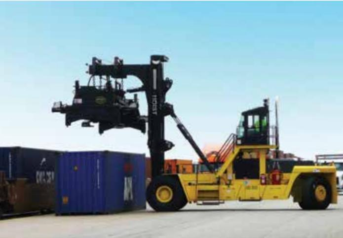
The LCH and ECH feature excellent all-around visibility with an elevated cab position, angled overhead window and wide-view mast. The unique mast design provides improved durability and reduced torsional stress. Various attachment options provide excellent serviceability and secure handling of loaded or empty ISO containers.
