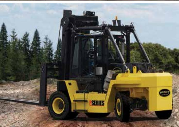
At competitive prices, heavy-duty grade RT utilizes premium components only suited for rough terrain, outdoor environments. The pneumatic tires are reinforced with all-wheel drive for better traction and control in uneven, outdoor environments, whether it be icy fields or unpredictable terrains in a military base.
