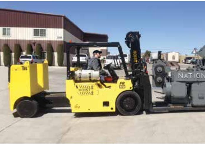
The innovative extendable counterweight frame is designed to provide stability at full capacity and extended load centers yet is compact enough for maneuvering in confined areas. Stackable counterweights and a removable hydraulic boom with collapsible boom stand allow for easy transport, while quick-change forks optimize performance.
