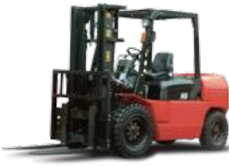
R series Diesel 4.0/4.5/5.0T PERKINS/NISSAN /LUOTO Engine
