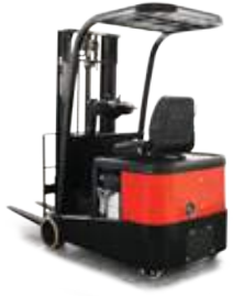
V series CPD10/12/15ET 1.0/1.2/1.5T AC ZAPI Controller
