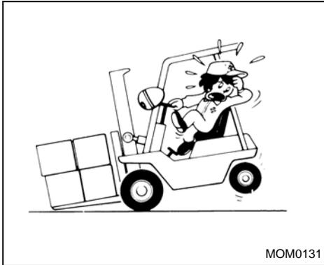
**!** Do not overload the forklift. Check the load chart for load weight and load center information. Always pick up loads as close to the center of the weight as possible to avoid off-center loading.
