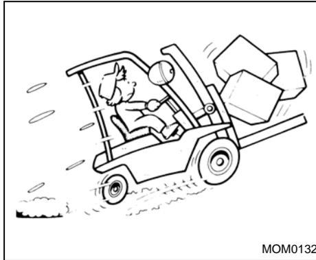
**!** Avoid sudden starts, stops or turns. Slow down for turns and on uneven or slippery surfaces that could cause the forklift to overturn or slide.
