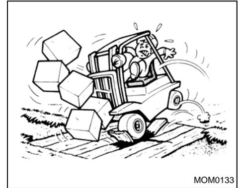
**!** Before driving over a dockboard or bridge plate, be certain that it is properly secured. Drive carefully and slowly across the dockboard or bridge plate. Never exceed its rated capacity.
