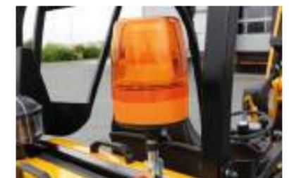
The optional rotating beacon is located in a protected position.
