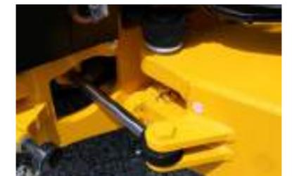
The articulated/swivel joint is maintenance-free and has an extended warranty.
